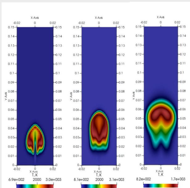
Fig. 2. Temperature distribution at  $t = 0.55$  ms (left); at  $t = 2$  ms (central); at  $t = 10$  ms (right)
