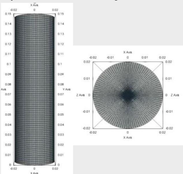
Fig.1. Mesh overlay on the research model using the OpenFOAM program
